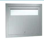
**0477** RECESSED TOILET SEAT COVER DISPENSER Door has tumbler lock, dispenses 500 single or half-fold seat covers. Wall Opening: 15%" x 111%" x 25%" (400 x 280 x 480 mm).
