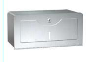
**0245-SS** PAPER TOWEL DISPENSER Dispenses 400 single-fold paper towel. Entire unit fabricated of 22 gauge stainless steel. Overall size:  $11\frac{14}{3} \times 6\frac{3}{3} \times 5\frac{5}{3}$  (285 x 160 x 145 mm).
